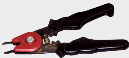
Designation Article no. MIG/MAG special gun Size 1, for 12-15 mm tips 1071000 Size 2, for 15-18 mm tips 1072000 ▶ Fast and dimensionally true cutting of the filler wire ▶ Time-saving cleaning and honing of the shield gas tip, and loosening and tightening the contact tip
