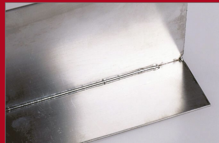
Welding Cr-Ni steel with TIG
