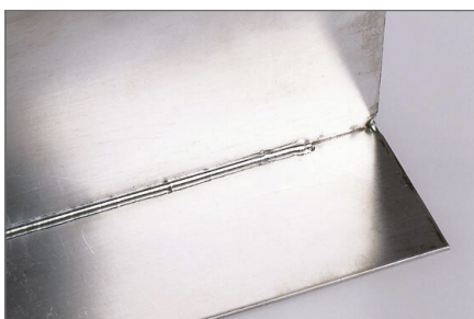
Welding Cr-Ni steel with TIG
